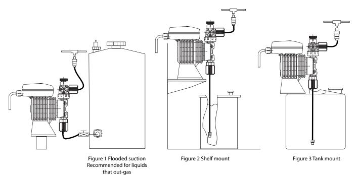
If flooded suction mounting is not possible, a shelf adjacent to (but not directly above) the supply tank often works well. (See Figure 2.) The supply tank or cover can also be used if it has provisions for mounting a pump. (See Figure 3.) In any case, the total suction lift should not exceed 5 ft (1.5m).
