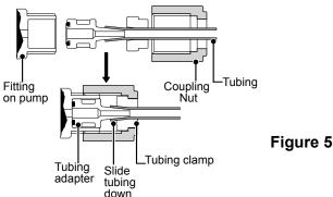
**WARNING:** All fittings and coupling nuts should be tightened by hand only. If necessary, a small tool may be used to make it snug. DO NOT use excessive force or large wrenches.
