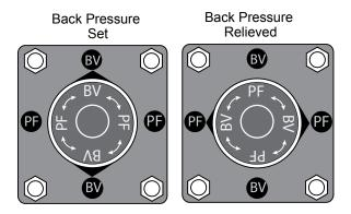
CAUTION: Confirm that liquid is discharged from the air vent drain. If the liquid is not discharged, the pressure may not be released. If this is the case, repeat the Pressure Relief procedure.
