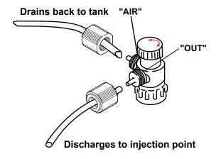
Figure 6 Air Vent Valve Tubing
