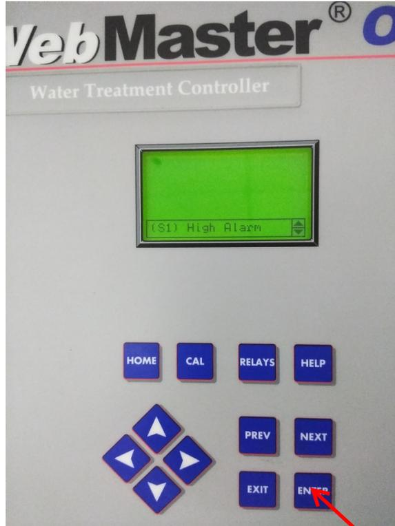
2. In the Main Menu, use the Previous and Next keys to navigate sub-menus until the Communication sub-menu is highlighted. Then press the Enter key.
