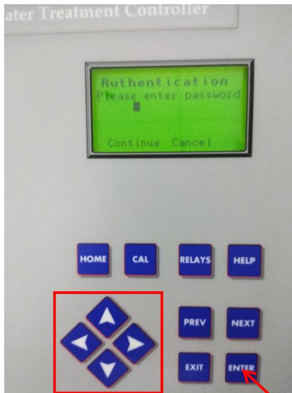
4. In the Communication sub-menu, use the Previous and Next keys to navigate until the ethernet IP address and ethernet subnet mask are visible on the screen. Make a note of these as they will be used in the direct ethernet connection procedure. The default IP address is 10.0.100.29 and the default subnet mask is 255.255.254.0.
