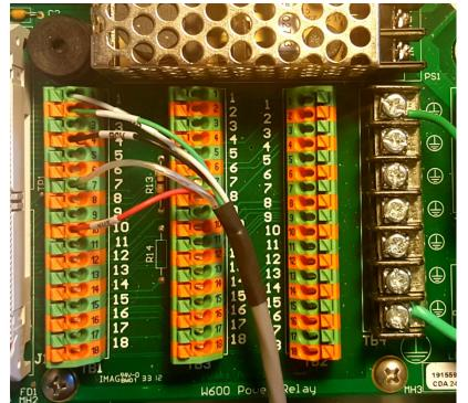
$\leftarrow$  The sensor wiring inside the controller.
