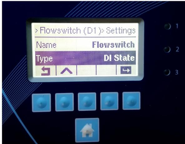
The Digital Input is now set up as an Interlock.
