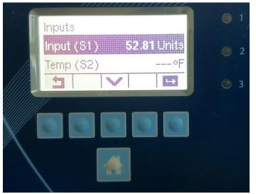
The W100 has only one sensor input. Input (S1) is for the sensor's reading, and Temp (S2) is for the temperature input (if the sensor has temp-comp). Press the ENTER Key to enter the Input (S1) menu. Press the Configuration Key X.
