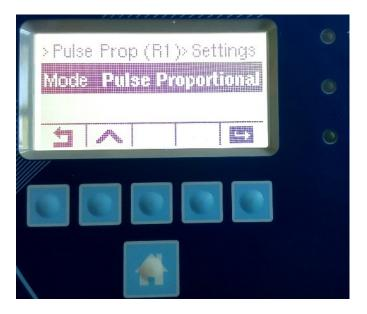
Use the Down Arrow  $\checkmark$  to scroll through the modes. Highlight the desired mode, and press the ENTER  $\checkmark$  to set the mode.
