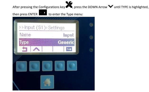
Once in the Type menu you can use the down arrow  $\checkmark$  to scroll through the sensor types. Select the desired sensor type and press the Check  $\checkmark$  to accept. You can also name the sensor in this menu.
