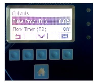
Press the **DOWN V** arrow to scroll through the 3 relay outputs.
