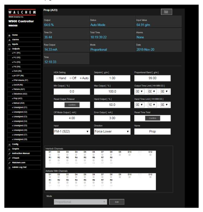
A22 = Disturbance Control; Primary Output = A23 (Proportional control based only on flow rate), Disturbance Input = V7 (ORP)
