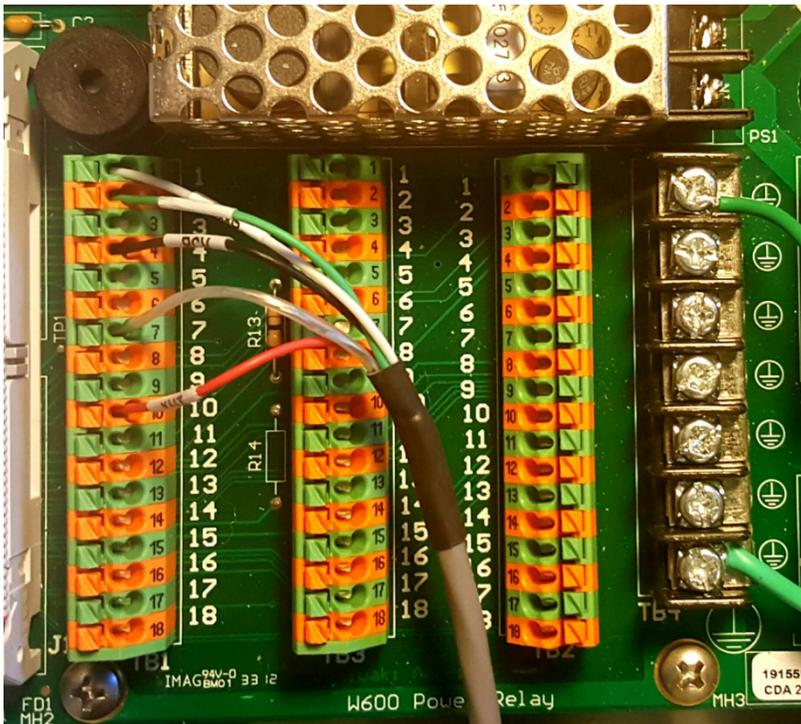
←The sensor wiring inside the controller.
