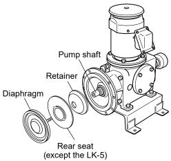
2. Fit the retainer and rear seat into the pump shaft and screw the diaphragm into the pump shaft. NOTE: The LK-5 does not have a rear seat. NOTE: Push down the retainer as far as
