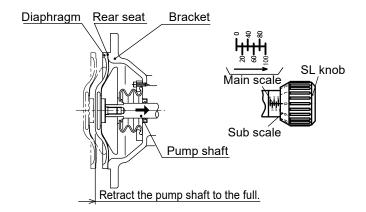
3. Set the stroke length to 100% and rotate the motor fan by the hand to retract the diaphragm to the full.
