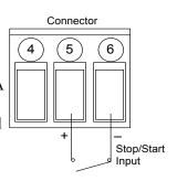
To connect the Stop/Start input from an external device, wire Terminals 5 and 6 from the contact closure. If using a solid state switching device, wire the connections ensuring that Terminal 5 is positive (+) and Terminal 6 is Common (-).
