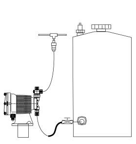
Figure 1 Flooded suction Recommended for liquids that out-gas
