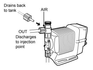
Figure 6 Air Vent Valve Tubing
