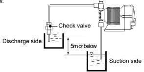
• A suction line pressure is higher than a discharge line pressure.
