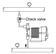
A discharge pressure (including pipe resistance and discharge head) is below 0.13MPa. (below 0.049MPa for B31 and C36).
