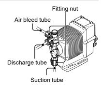
3 Remove the pump head with a hexagon wrench.
