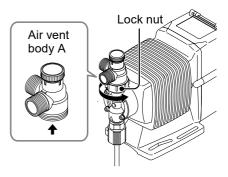
3 Remove the air vent body B by the 0.9inch (21mm) box wrench.
