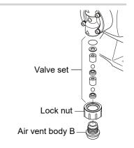
3 Connect the flow checker body and the pump head with the Lock nut. Turn the Lock nut anticlockwise to tighten them. Take care not to drop the Plate, O ring or Float. Note that the Float has a mounting direction. Install the float into the body with a red-marked face upwards.
