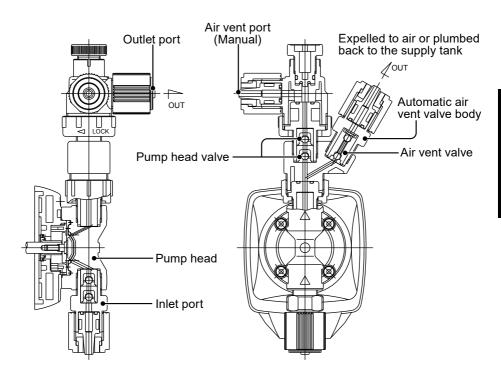
The lower opening pressure (open air pressure) of the auto vent valves than the outlet check valves lead the entrained gas to the open air via the branched air vent route. Once all gas in the pump head is expelled, liquid starts to flow the main path to the outlet.
