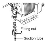
Remove the fitting by an adjustable wrench or a spanner.
