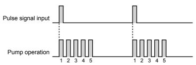
A buffer works when the pump receives an external pulse before the set shots per signal is completed. The buffer is active with the factory default settings.
