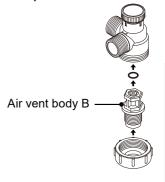
4 Pull out the valve set by a pair of tweezers.
