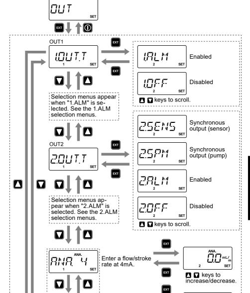
Enter a flow/stroke rate at 20mA.
