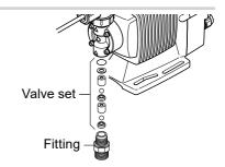
2 Place the valve set into the air vent body B and tighten it into the pump head to 3.5N·m through the Lock nut.
