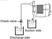
• A discharge side liquid level is higher than a suction side but the distance is 5m or below.
