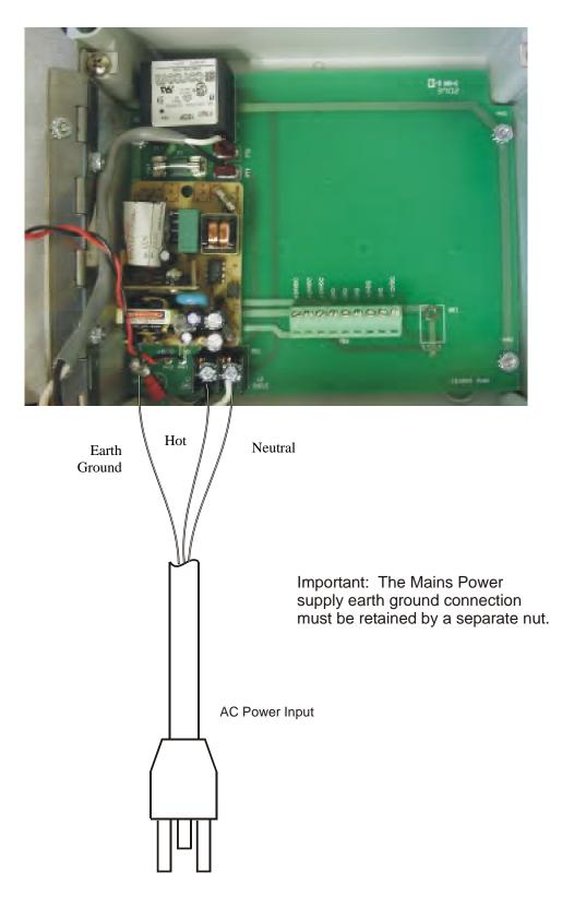
Figure 2 – Wiring Diagram for AC Power Input
