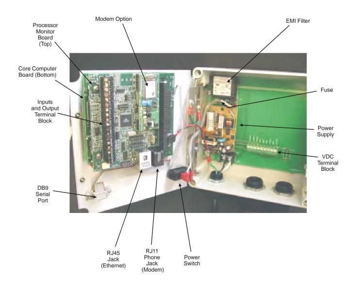
Figure 1 Identification of Parts
