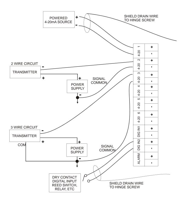
Figure 3 - Wiring Diagram for Inputs, Externally Powered
