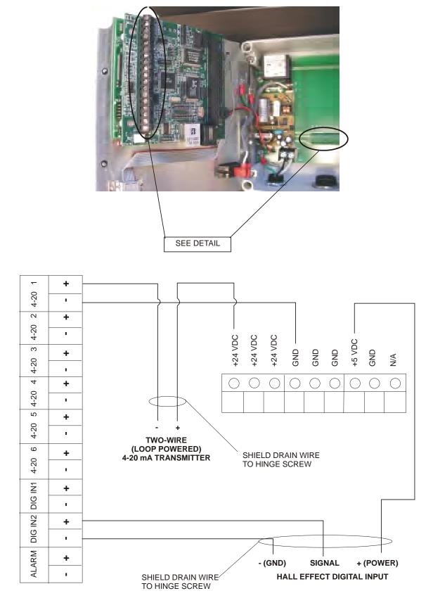
Figure 4 - Wiring Diagram for Inputs, Powered by WebAlert
