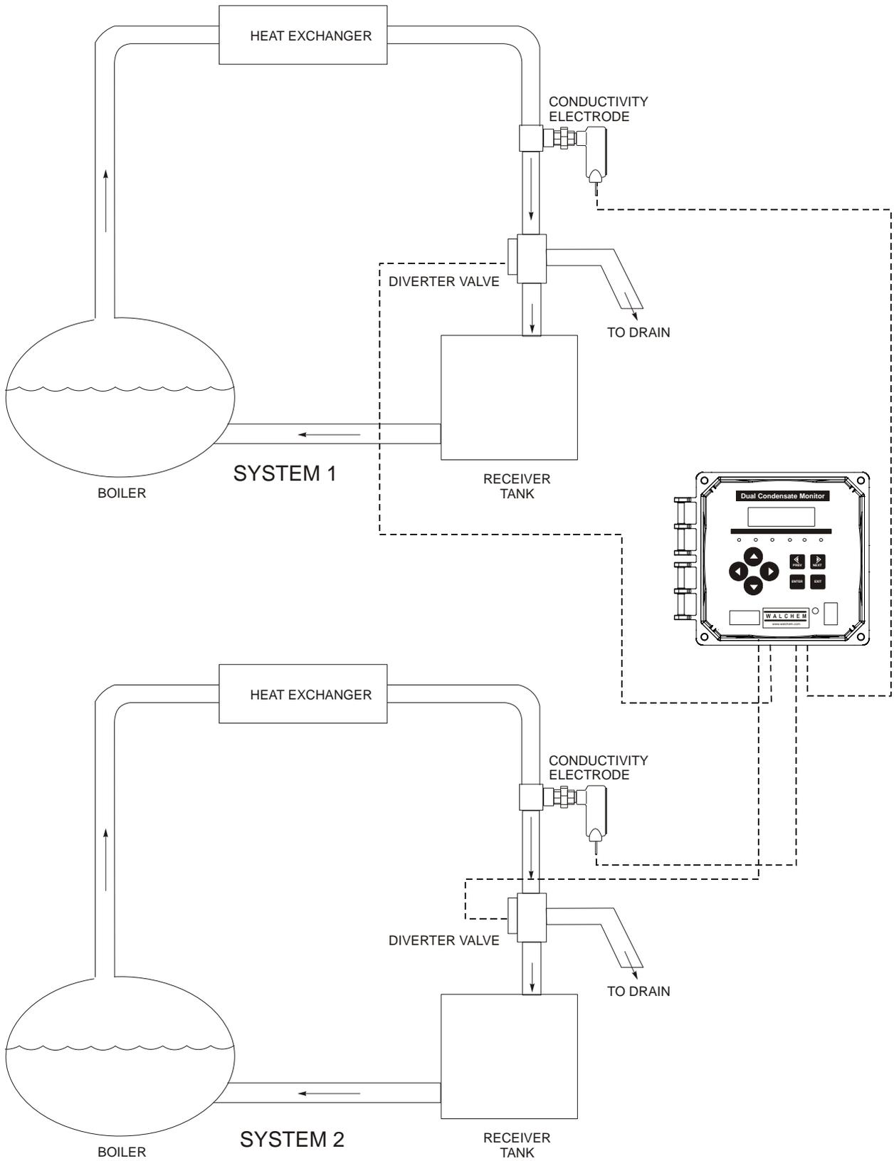
**Figure 2 Typical Installation**
