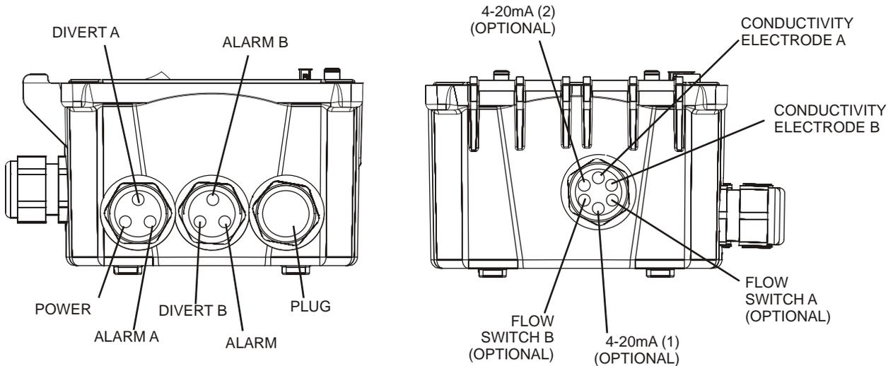
**Figure 1 Conduit/Wiring Configuration**
