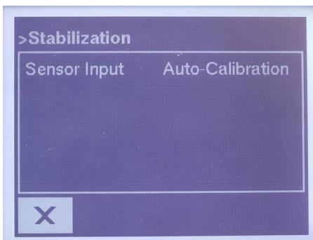
This screen shows "Auto Calibration" for a few seconds for Sensor Input, and then it will show a mV reading during this Stabilization process. Once the reading is stable, it will **automatically** go to the next screen.
