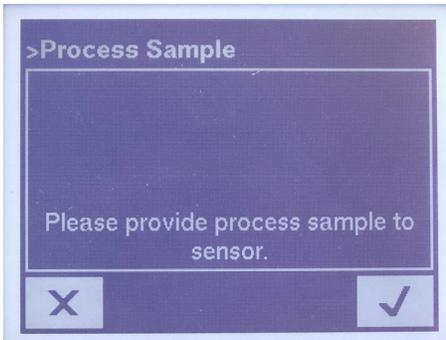
Remove water sample and rinse or blow out tube to ensure good sample reading. Add process sample and **wait 4 minutes** before pressing ✓
