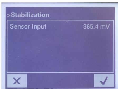
This screen shows “Auto Calibration” for a few seconds for Sensor Input, and then it will show an mV reading during this Stabilization process. Once the reading is stable, it will **automatically** goto the next screen.
