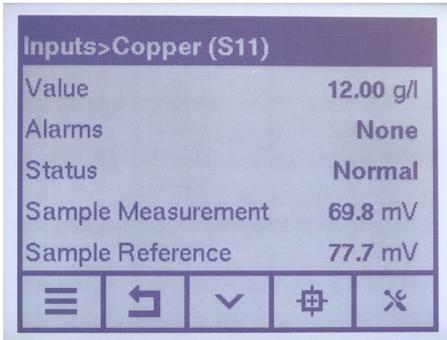
This screen is displayed once Water/Sample Calibration process is complete and control is resumed. The **Sample** Measurement and Reference numbers are displayed. Press the down arrow to review the **Water** Measurement and reference calibration numbers that were saved during Water/Sample calibration.
