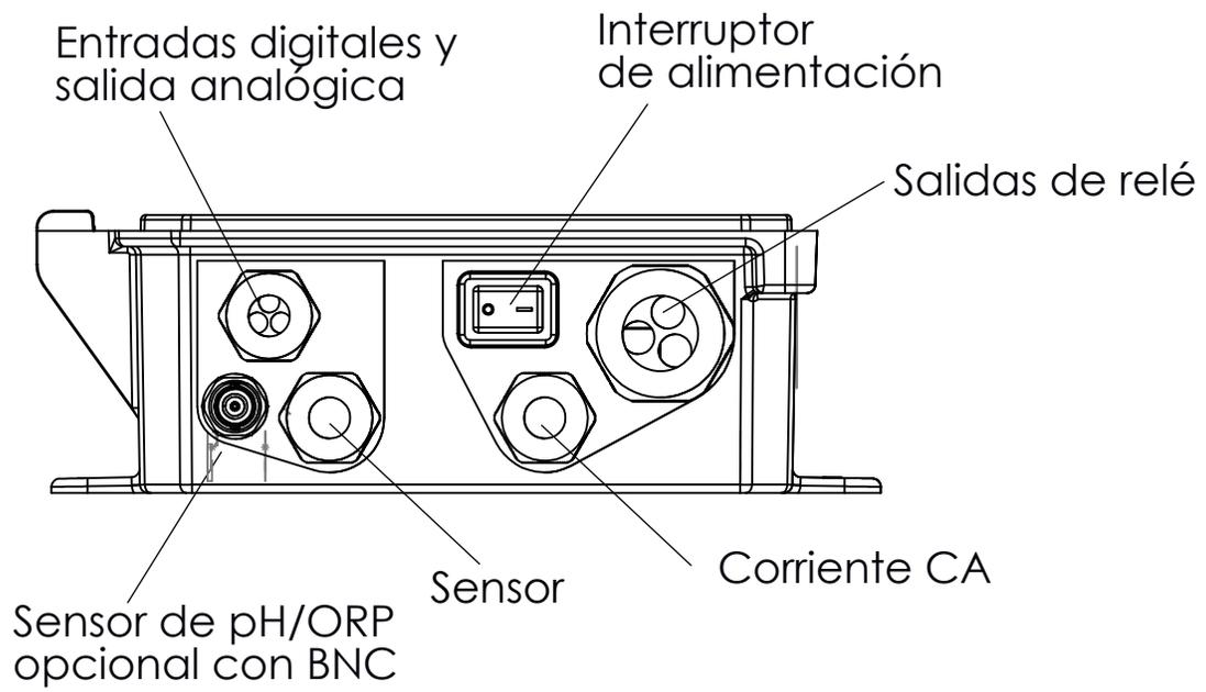
**Figura 1 Cableado**
