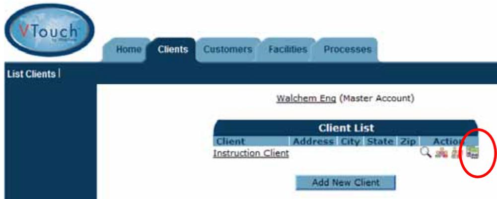
You will be presented with a list of all controllers that are assigned to that client. Any unassigned controllers will be listed at the bottom. Locate the serial number of the controller to be assigned, and then click on the Assign button.
