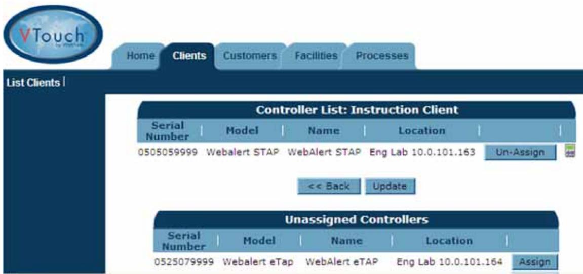
Click The Customers tab (or the next tab down) and repeat the process of assigning the controller to the desired Customer level company, and Facility level company.
