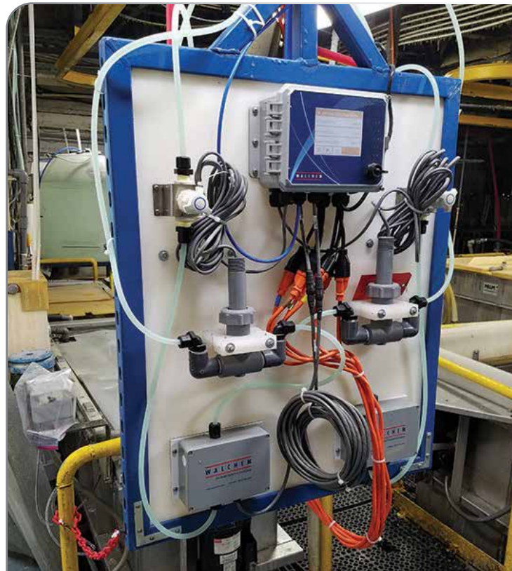
WNI600 Series Electroless Nickel controller manufactured by Walchem - IWAKI America Inc. Photo Credit: IWAKI America Inc.
