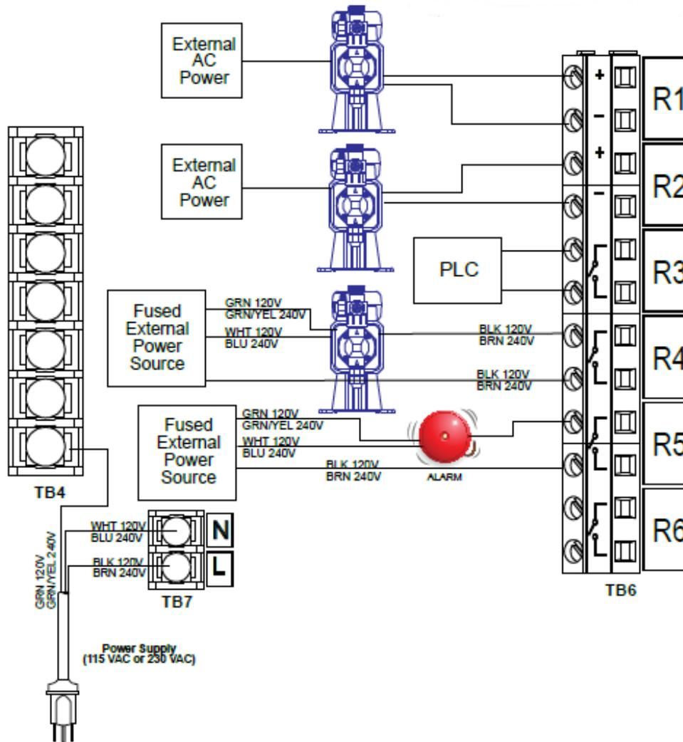
Figure 16 W620 AC Power & Relay Output Wiring
