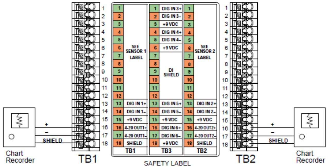
Figure 18 Analog Output Wiring
