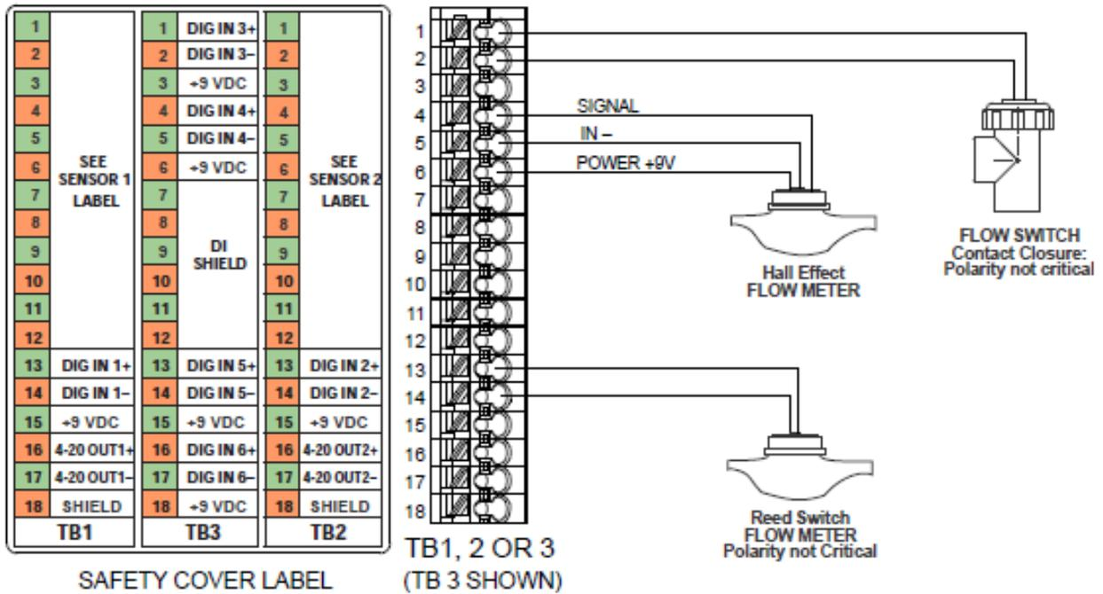
Figure 13 Digital Input Wiring
