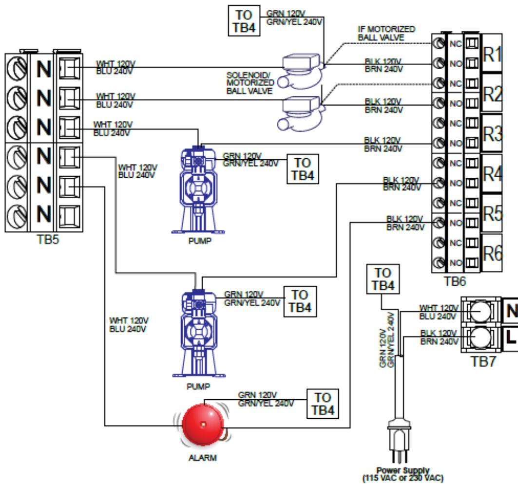
Figure 14 W600 AC Power & Relay Output Wiring
