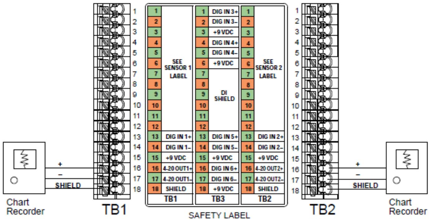
Figure 18 Analog Output Wiring
