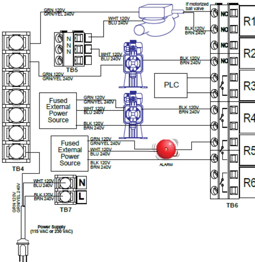
Figure 15 W610 AC Power & Relay Output Wiring
