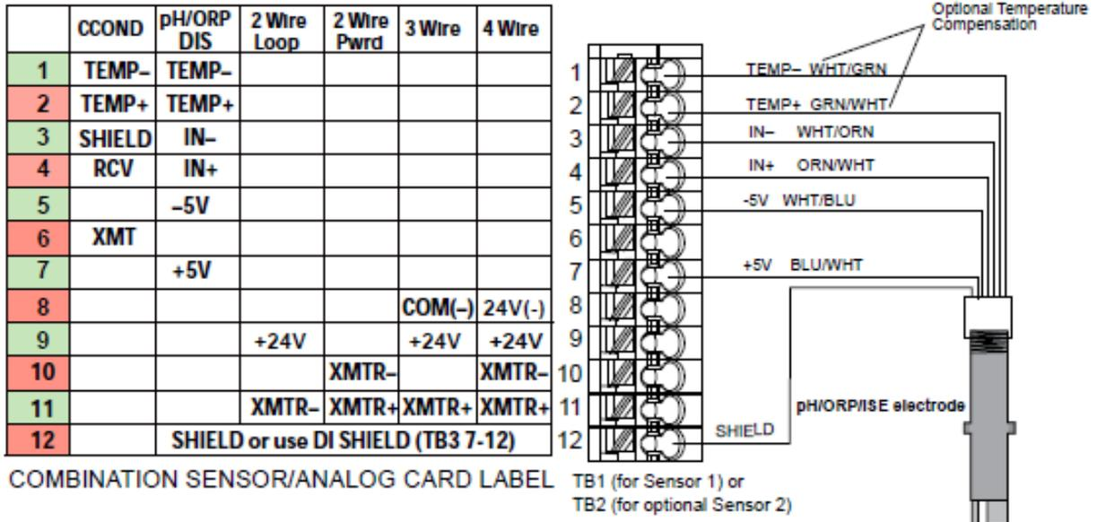
Figure 9 pH/ORP/ISE Sensor Input Wiring
