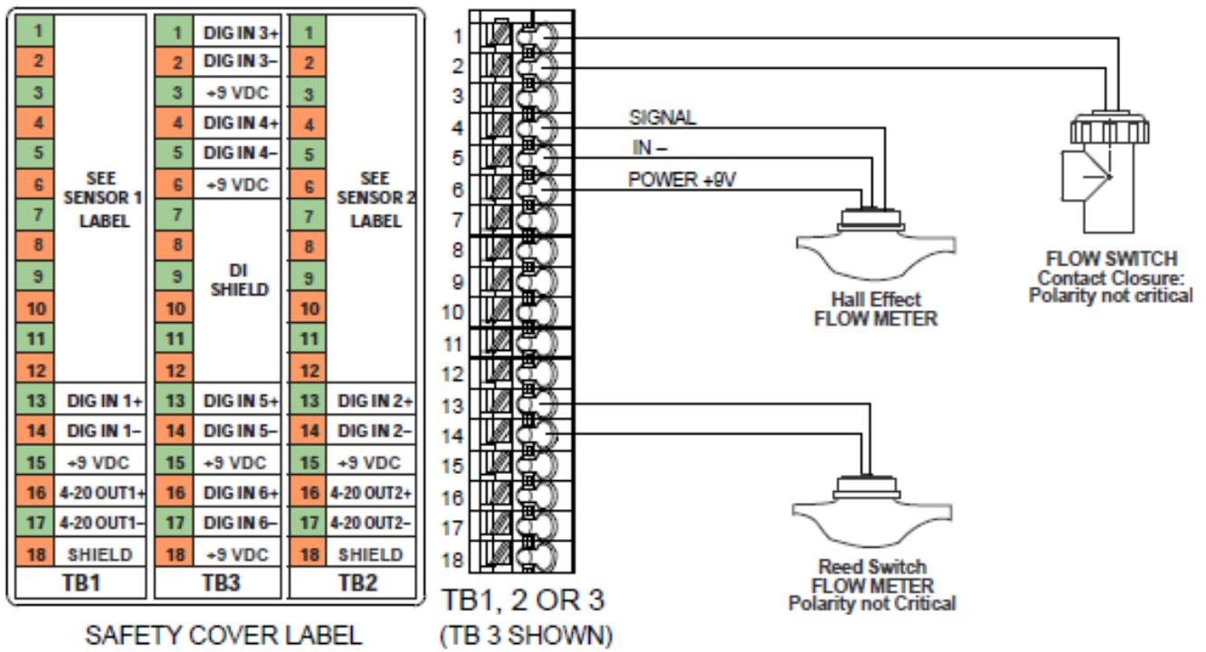
Figure 13 Digital Input Wiring
