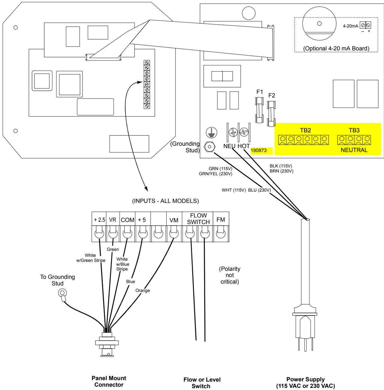
Figure 3a Inputs (for power relay board #190873)
