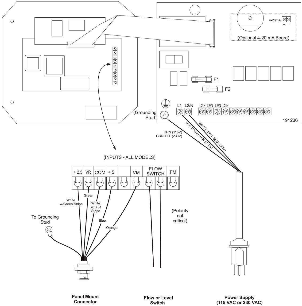
Figure 3 Inputs (for power relay board #191236)
