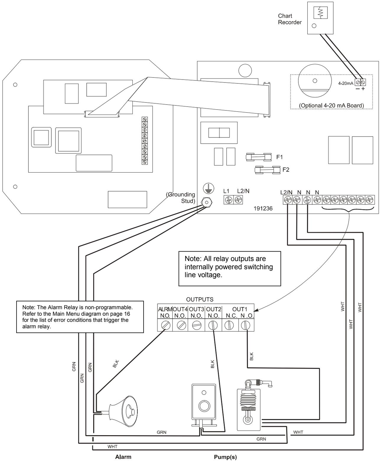
Figure 4 Outputs (for power relay board #191236)
