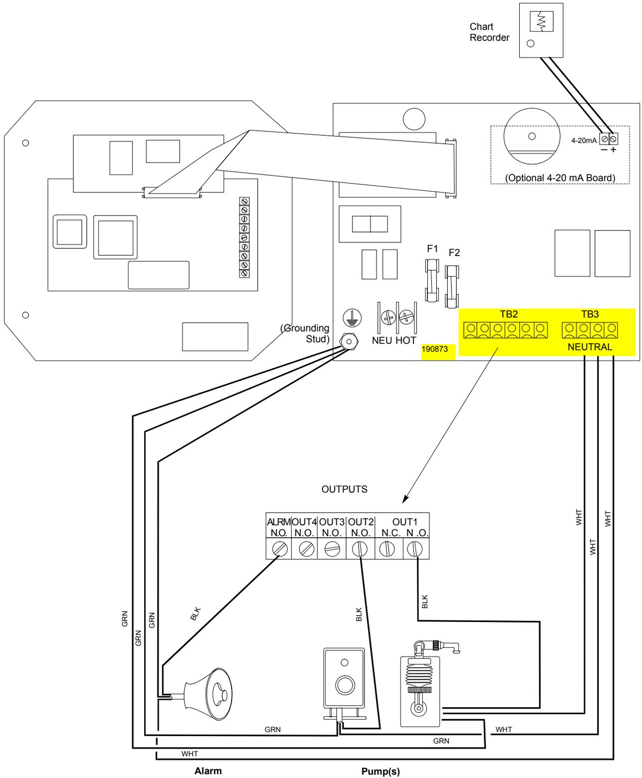
Figure 4a Outputs (for power relay board #190873)
