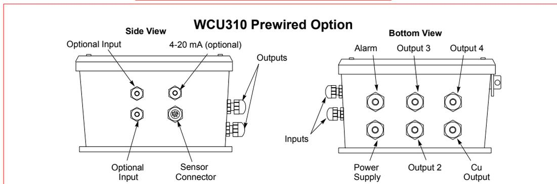
Figure 2 Conduit/Wiring Configuration
