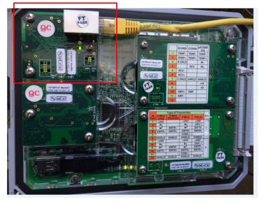
Ethernet is standard in a W900 controller. Open the controller front door, and on the backside, bottom center, you will find the Ethernet RJ45 port.
