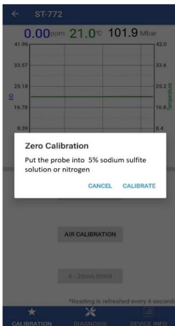
Figure 8 Zero calibration
