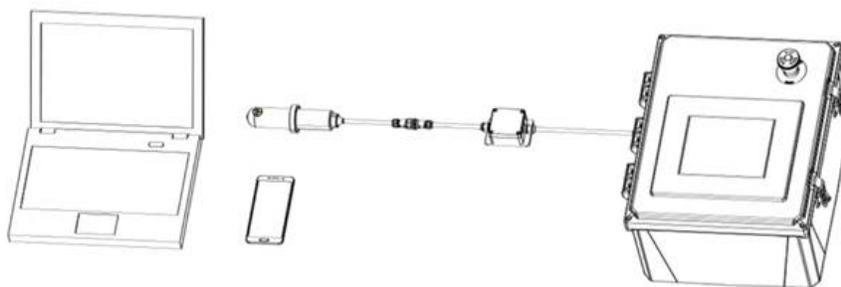
**Figure 5.** Bluetooth connection to ST-500 Series sensor
