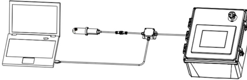
Figure 6. USB connection to ST-500 Series sensor
