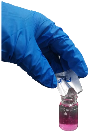
Figure 3. Add DPD powder to the 10 ml sample vial
