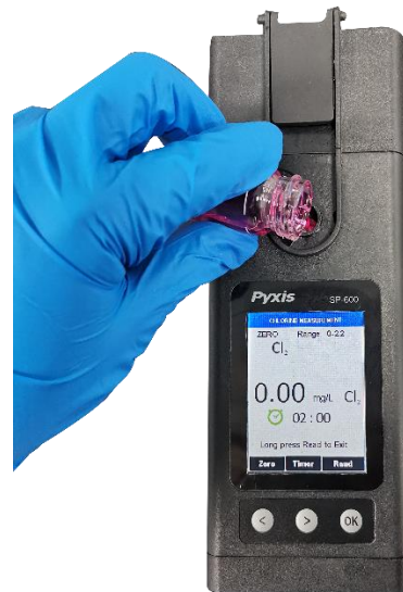
Figure 4. Transfer the developed sample to sample cell
