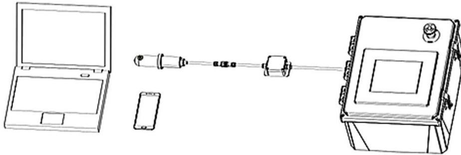
Figure 4. ST-500 connected to computer via USB-485 adapter
