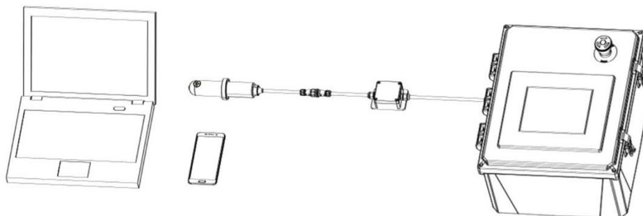
Figure 3. ST-500 connected to computer or smart phone via WiFi/Bluetooth adapter
