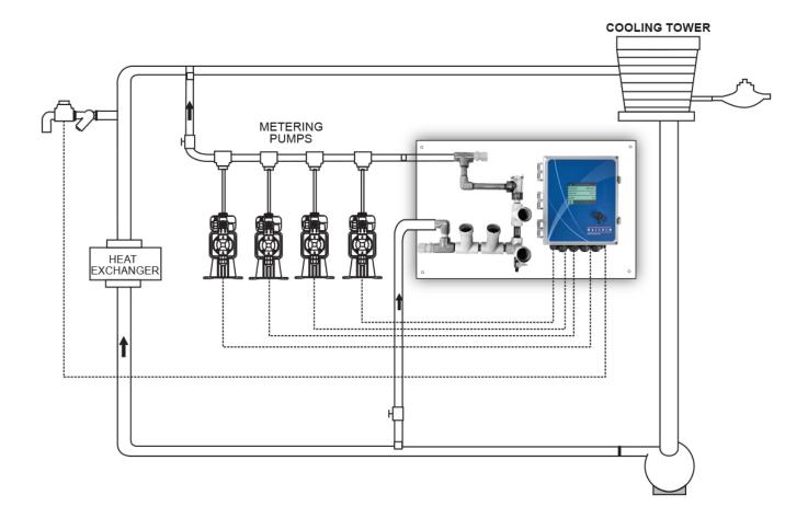
Figure 1 Typical Installation
