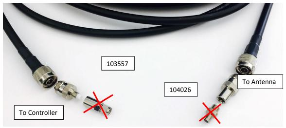
Remove the 103557 from one end and the 104026 from the other end prior to installing the extension cable.
