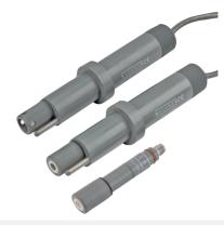
The WEL Series are modular in design with a rugged CPVC housing that contains the electronics. pH and ORP cartridges can easily be connected or replaced in minutes without tools. The cartridges feature a unique threaded interlock connection and a double o-ring seal, ensuring a watertight fit and secure seating at all times.
