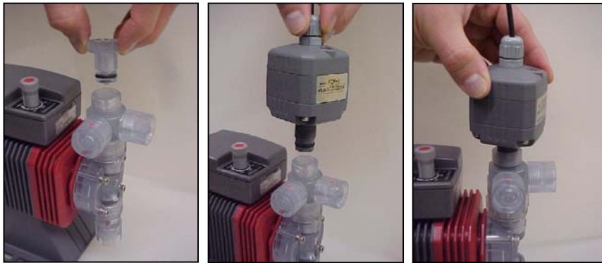
Installing the PosiFlow ® Sensor into the manual air vent valve.
